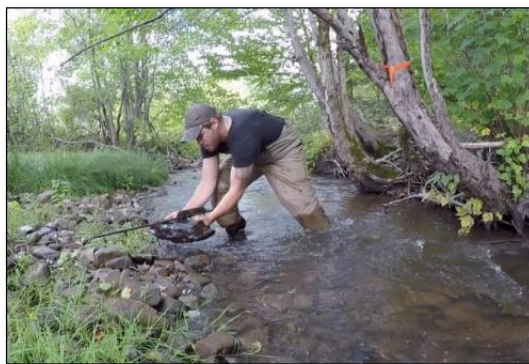
Figure 26: Installation of a water temperature logger in-stream
