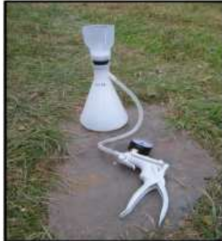
Figure 2: Water filtering equipment assembly: Taken from “eDNA protocol sample collection, Goldberg & Strickler, 2015, Washington State University”.
