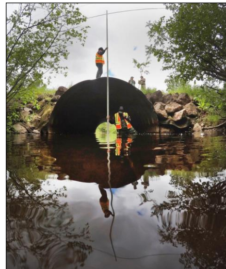
Figure 9: SBWA during a culvert assessment survey
