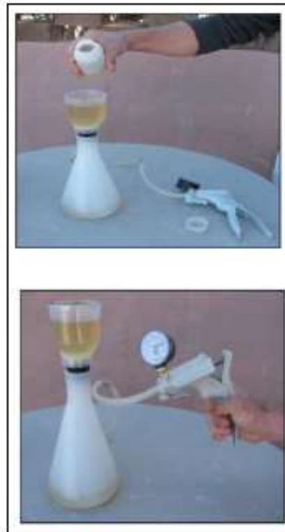
Figure 4: Water filtration illustration: Taken from “eDNA protocol sample collection, Goldberg & Strickler, 2015, Washington State University”.
