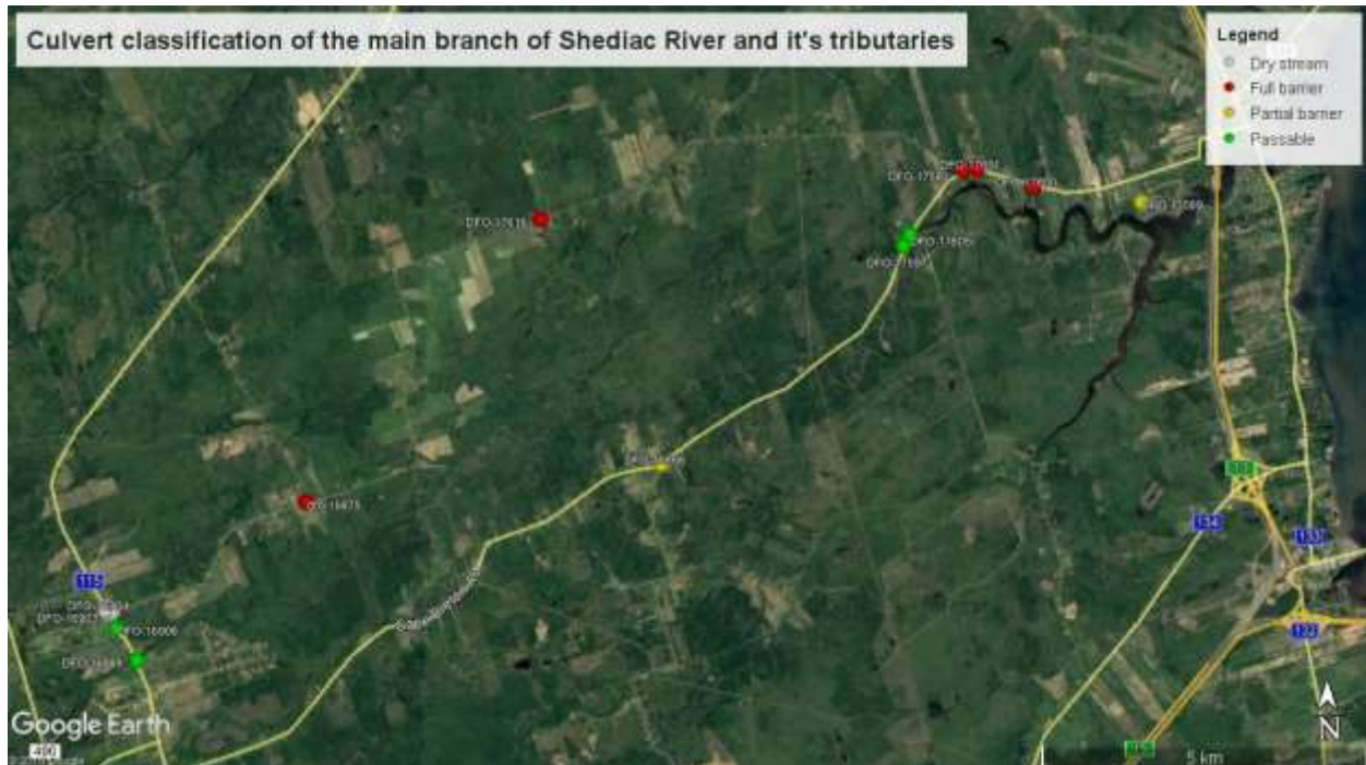
Figure 46: Culvert classification for the Shediac River, 2018
